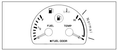
The engine coolant temperature and fuel gauge
