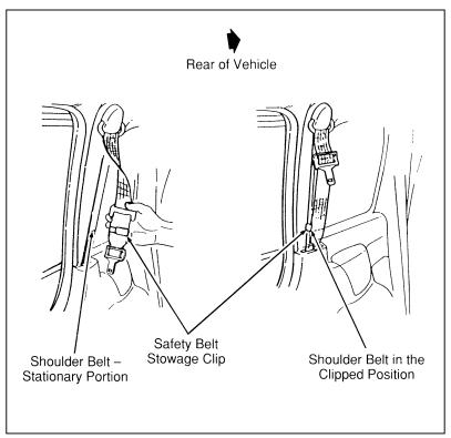
Figure 2: Securing the detachable shoulder belt
