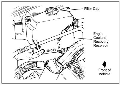
Engine coolant recovery reservoir fill location
