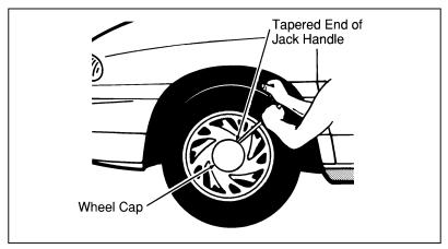
Wheel cover removal (optional cast aluminum wheels)
