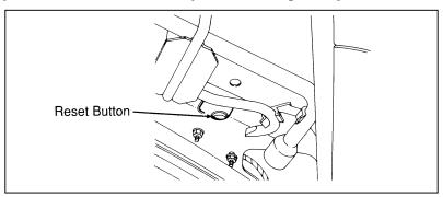
Fuel pump shut-off switch reset button location
