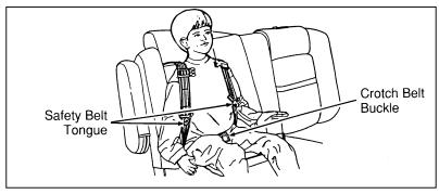
Figure 4: Shoulder safety belt placement on the child
