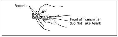
Replacing the batteries
