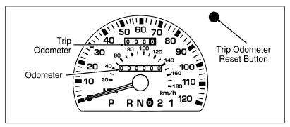
The speedometer, odometer and trip odometer
