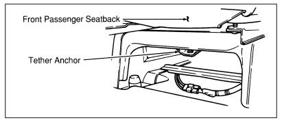
Figure 1: Tether anchor location — Front passenger seat
