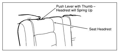
Figure 1: Releasing the headrest
