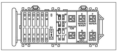
Engine compartment main fuse and relay panel
