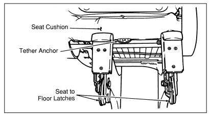
Figure 4: Tether anchor location — second row bucket seat
