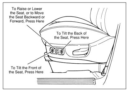
The power controls on the driver's seat
