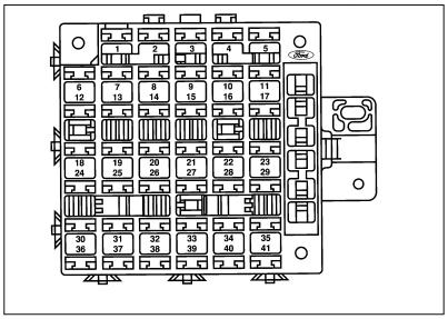
Main fuse panel under instrument panel
