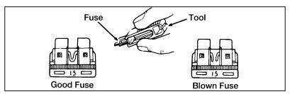
Fuse puller tool and fuse
