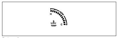
Engine coolant temperature gauge
