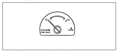
Engine coolant temperature gauge — base cluster
