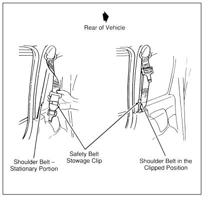
Figure 2: Securing the detachable shoulder belt
