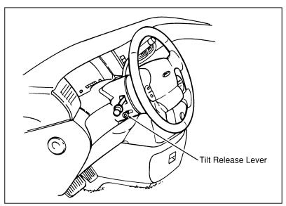
Tilt steering release lever location
