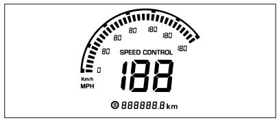
The speedometer and odometer
