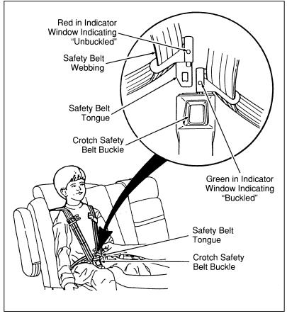
Figure 5: Fastening the crotch safety belt buckle
