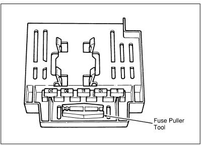
Fuse puller tool location — fuse panel cover
