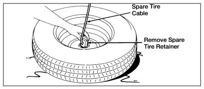
Removing the spare tire retainer
