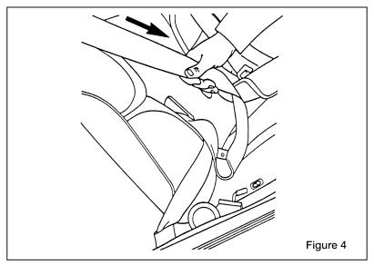
Setting the retractor to automatic locking mode
