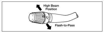
High beam and flash-to-pass operation
