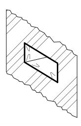
New radios 'DIN' cage slid into the 'DIN' opening of the dash with its tabs bent securing the cage to the dash.
